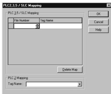
A Logix 5000™ controller stores tag names on the controller so that other devices can read or write data without having to know physical memory locations. Many products only understand PLC/SLC data tables, so the Logix 5000 controller offers a PLC/SLC mapping function that lets you map Logix tag names to memory locations.
